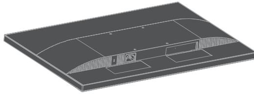
Step 4: Attach the mounting bracket from the VESA compatible wall mounting kit (100mm x100mm distance), VESA Mounting Screw M4 x 10 mm.
