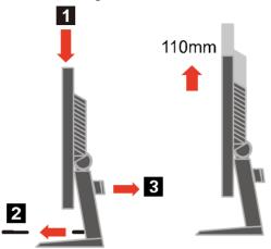
2> Insert the L bracket to the base metal plate; Remove the cable manager and put the monitor flat on the desk.
