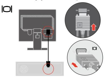
Connect the digital cable to the DVI connector of the monitor and the other end on the back of the computer.
