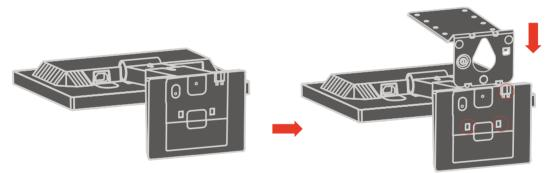
3> Tighten the quick release screw with L bracket; Fix U chip on the L bracket.
