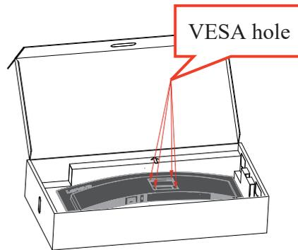
Step 5: Attach the LCD display to the wall, and follow the instructions in the wall-mounting kit.
