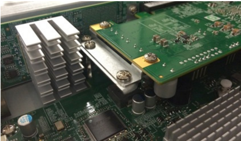
Figure 6-10. Installing the Internal Expansion Card
