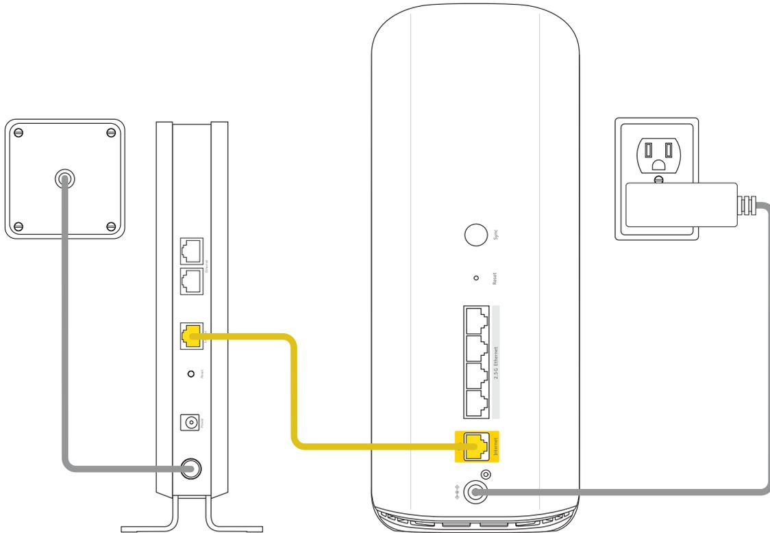
Figure 3. Connect the router to a modem
